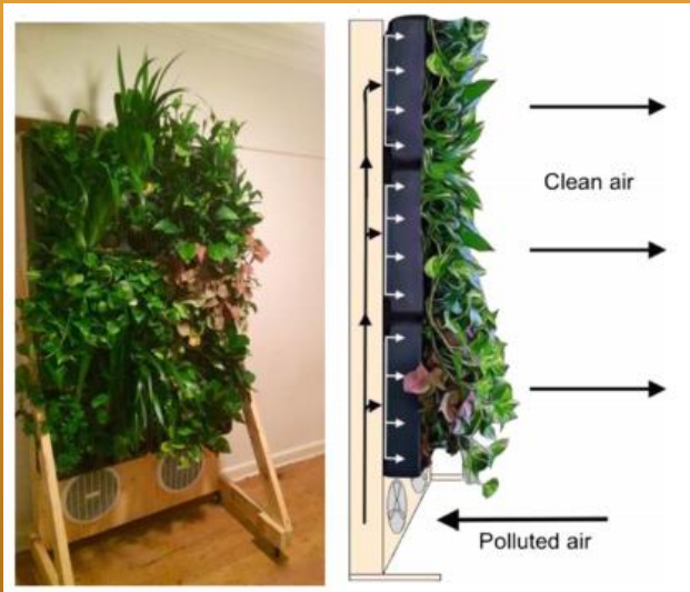
Figure 1. Diagram of active green wall (AGW) functionality (Pettit et al. 2018a).
